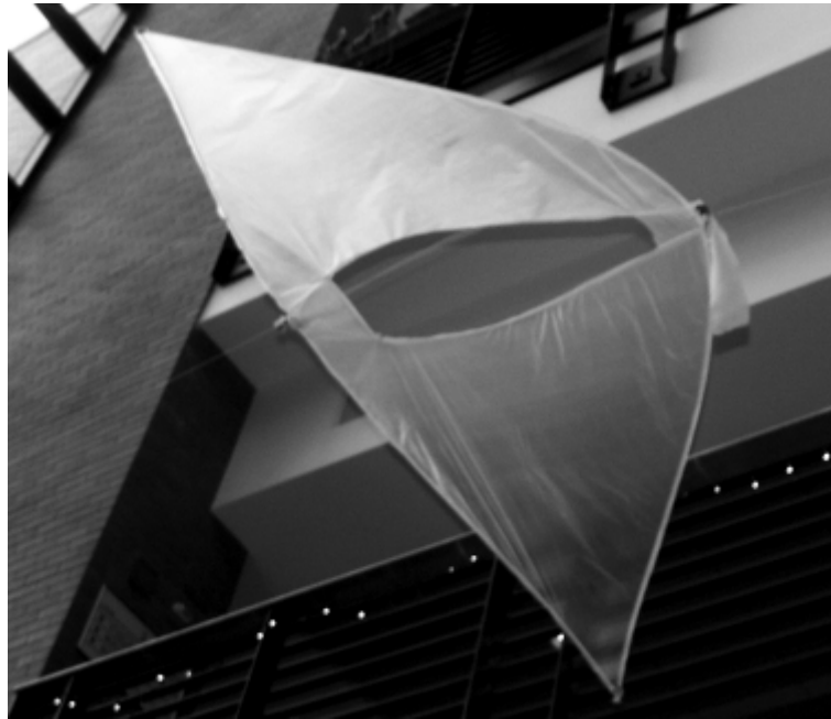
Fig. 1. A view of the kite-like Manta ray suspended from computer-controlled fishing lines in the three-story atrium of Rochester Institute of Technology's B. Thomas Golisano College of Computing and Information Sciences. The manta is comprised of fiberglass rods with a translucent skin upon which we can project digital images. Because the rods are joined in a state of dynamic tension, they flex and bend when the lines are moved, producing a lifelike swimming motion.
